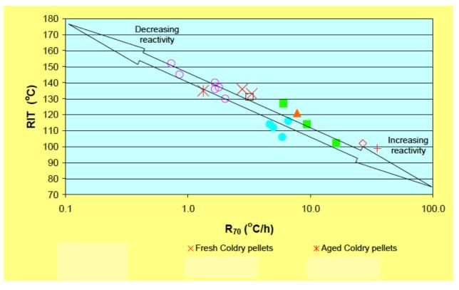
Figure 2 – Relative Ignition Temperature vs. R<sub>70</sub> (rate of self heating)
