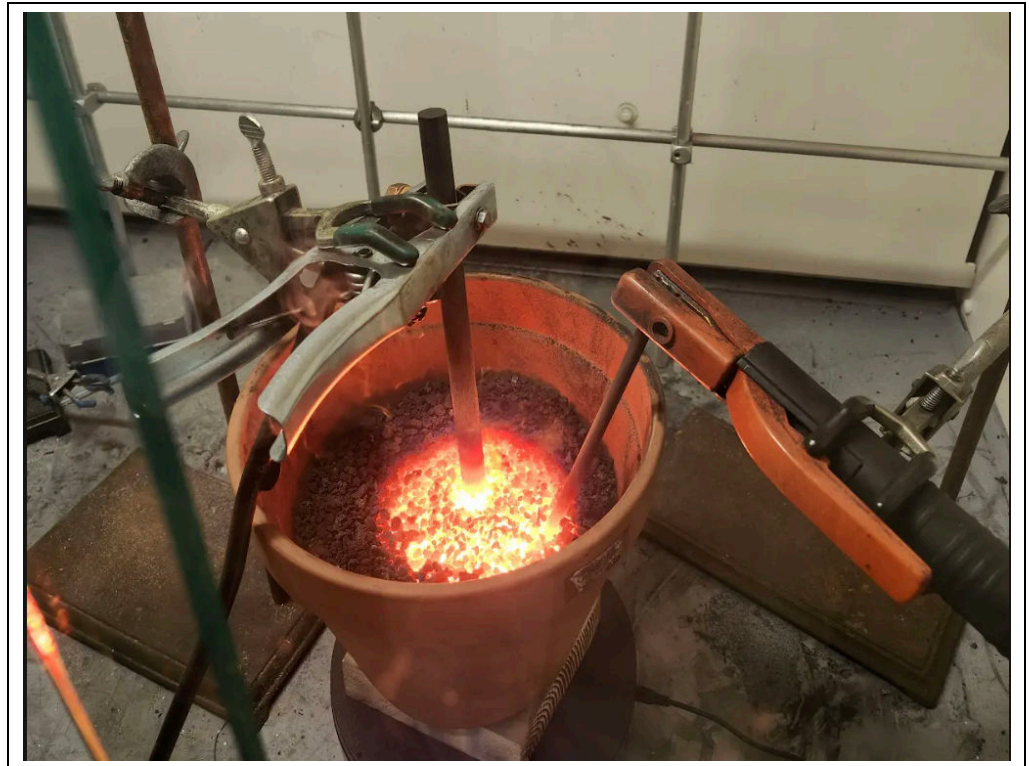
Figure 2: ECT initial lab testing of FJH with small soil sample size
